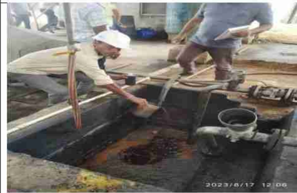
Photo 3: Spent wash sampling from MEE section in molasses plant
