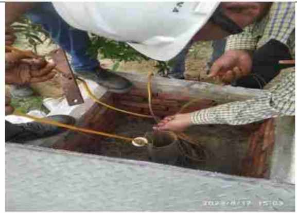
Photo 13: Sample collection from Piezo well in grain plant
